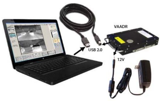
VAADR is plug-and-play capable with USB2.0. Just plug it in to any PC or laptop, and have instant access to all video on the drive.
